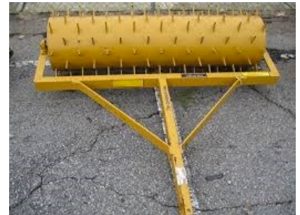
A common design for an aerator is a roller wheel with spikes designed to puncture
