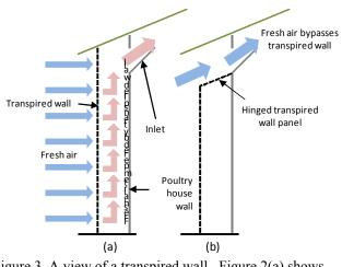
Figure 3. A view of a transpired wall. Figure 2(a) shows fresh air being tempered by the transpired wall and figure 3(b) shows the fresh air bypassing the transpired wall for mild weather ventilation.
