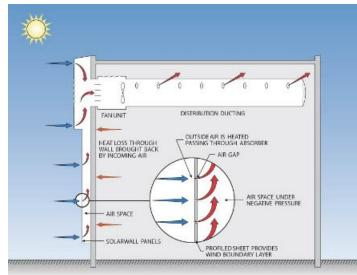
Figure 2. How the transpired wall works at the INTEK facility in Aberdeen, NC
