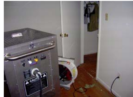
Heat treatment of an infested apartment.
