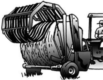
One last very important tip for machinery is to keep a dry chemical fire extinguisher on the tractor. Heat can build up due to friction created by contact of dry hay or forage material with faulty bearings and baler belts. Farmers report that this friction and overheating has caused bales to ignite. People have been burned trying to deal with a baler fire.
