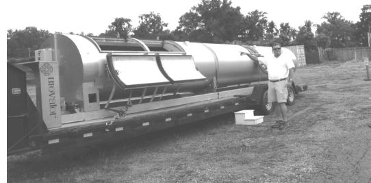
Henry Moore shows a Biovator unit, one type of commercially available in-vessel composting system. These systems rotate the materials providing increased aeration which speeds up the composting process and eliminates the need for turning by hand or loader.
