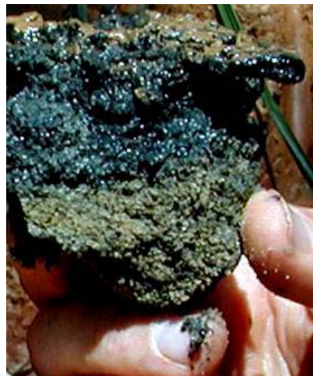
Figure 1. Biomat from trench bottom. Thickness of dark material is about 3 cm.
