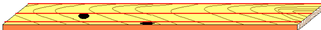
b) locating strips with regard to the parts obtained, and locating the knot in only one strip.
