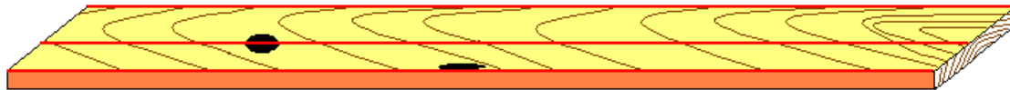
a) filling the width of the board with usable strips, and splitting the knot between strips.
