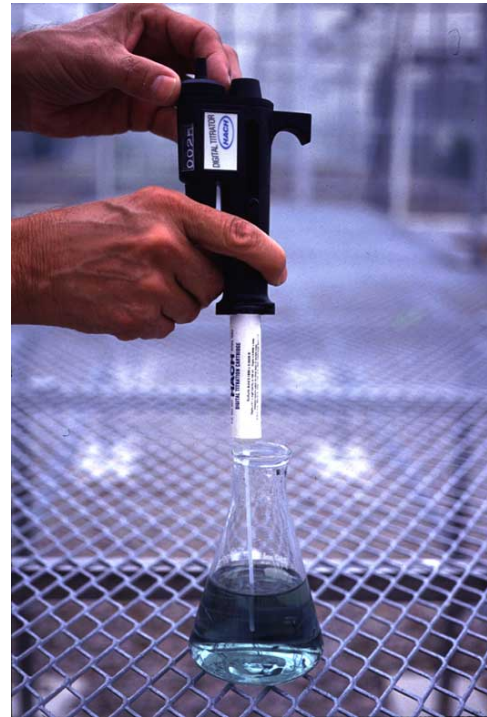
Alkalinity is measured by adding an indicator dye to a sample, then titrating with an acid until the solution changes color.
