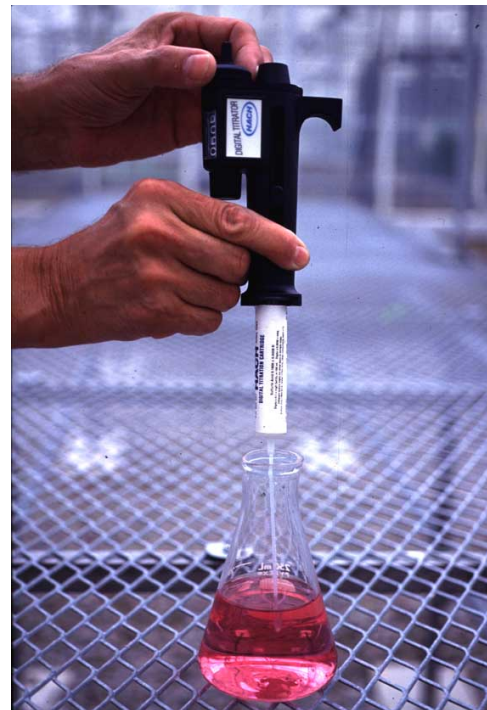
The indicator dye in this kit turns from green to pink when all of the alkalinity has been neutralized (at pH ~4.6). The alkalinity of the solution equals the meq of acid required to reach the endpoint color change.
