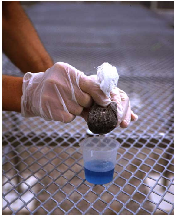
Combined plug samples are placed into cheesecloth, and the substrate is collected for analysis. Plastic gloves prevent solution contamination from your hands.
